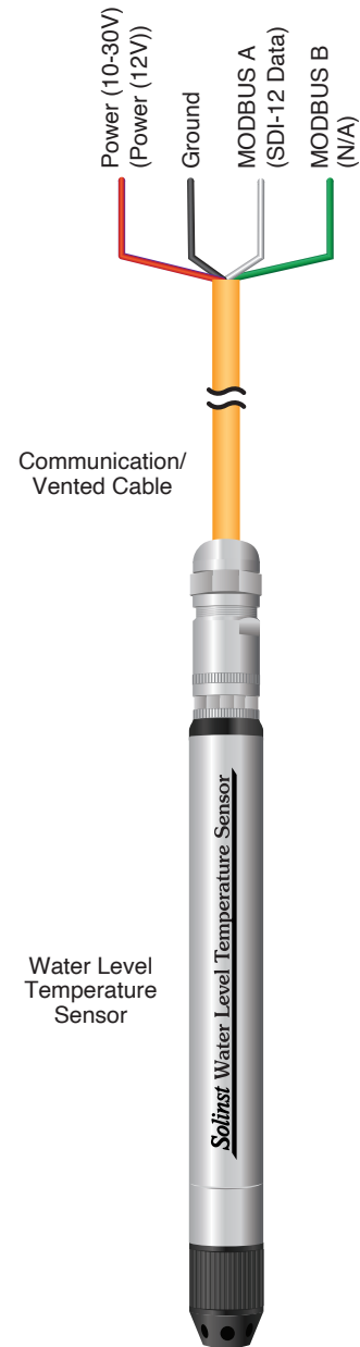
MODBUS Wiring Overview (SDI-12 in Brackets)
